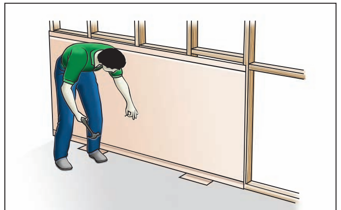
FIGURE 4 FIXING FIRST SHEET
