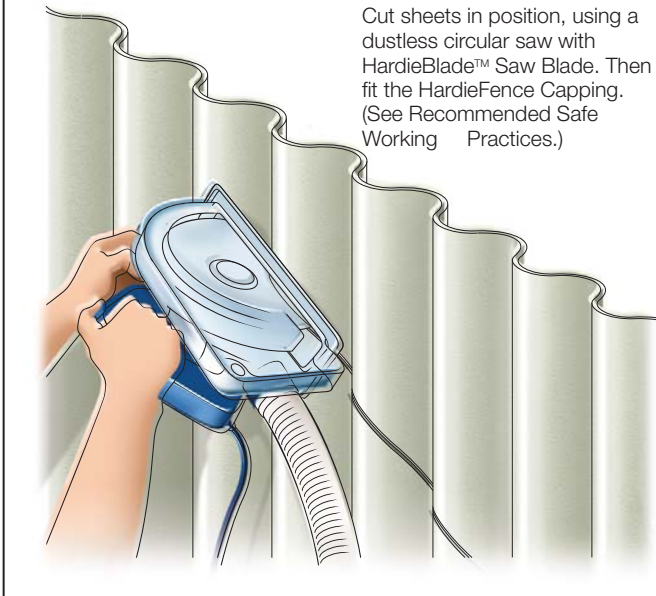
FIGURE 11 HARDIEFENCE SHEETS MAY BE CUT ON A RAKE
